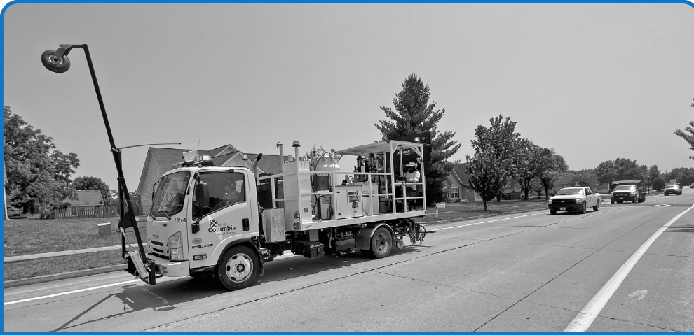
A striping truck, which drives in a procession due to the time required for the paint to dry. Never attempt to pass a line of striping trucks—instead, use the next intersection to find an alternate route.
