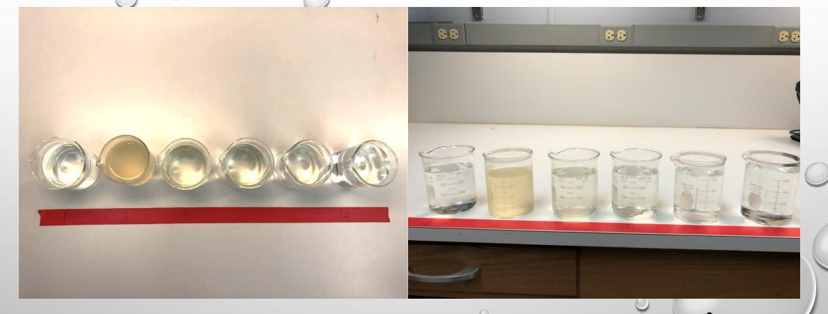
1<sup>ST</sup> GLASS RAW WATER, 2<sup>ND</sup> GLASS AERATOR EFFLUENT, 3<sup>RD</sup> GLASS PRIMARY EFFLUENT, 4<sup>TH</sup> GLASS SECONDARY EFFLUENT, 5<sup>TH</sup> GLASS FILTER INFLUENT, AND 6<sup>TH</sup> GLASS FINISHED WATER
