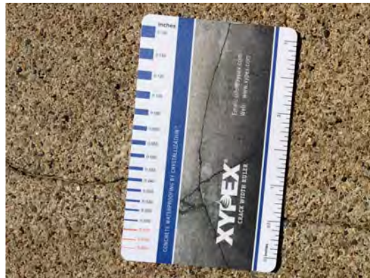
Crack Comparator Measurement at Top of Wall.
