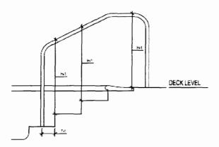
7.7.5 <u>Deep Water</u> - Where stairs are provided in swimming pool water depths greater than five feet (1.5 m), they shall be recessed and not protrude into the swimming area of the pool. The lowest tread shall be not less than four feet (1.2 m) below normal water elevation.
