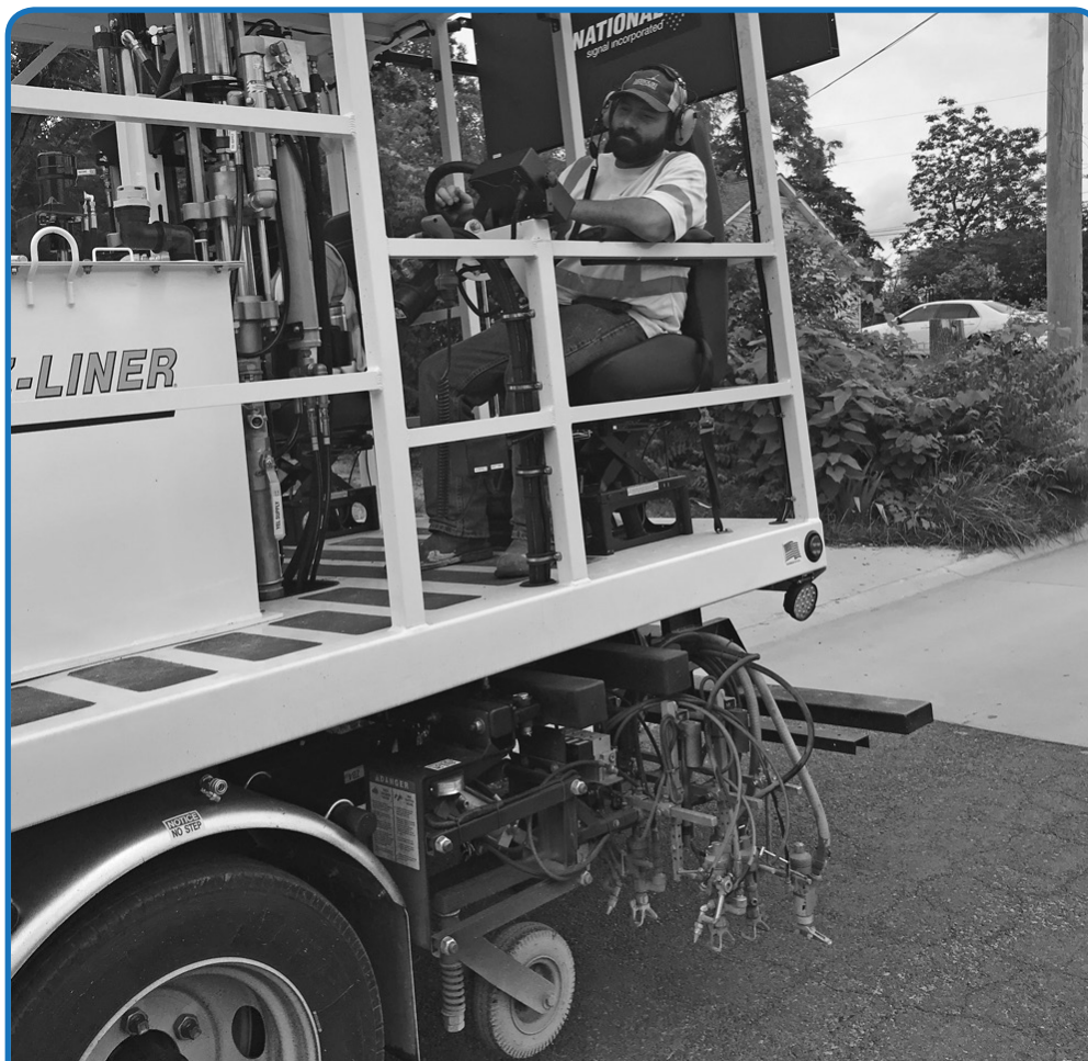
The City's new line striper uses MoDOT-approved Type P retroreflective paint with glass beads that turns the light around and sends it back in the direction of drivers' headlights.
