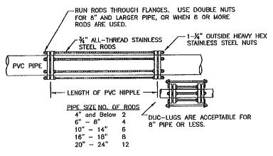
TIEBACK RODS MAY BE ATTACHED TO D.I. FITTINGS, VALVES, HYDRANTS, AND CONCRETE RESTRAINING BLOCKS.
