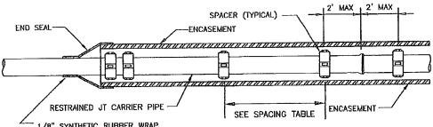
1/8" Synthetic Rubber Wrap Around end Seal With Stainless Steel Banding Straps
