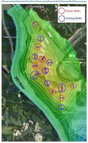
Options were considered for expanding existing well fields. Existing and potential sites for future wells are highlighted in the figure above.
