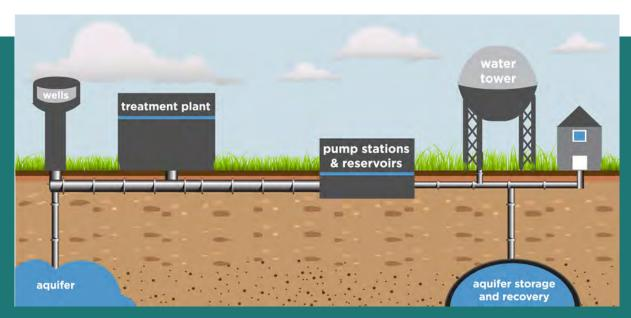
Columbia's water is pumped from 15 wells that tap an alluvial aquifer in McBaine, MO. Softened, filtered, and disinfected water is pumped from the treatment plant to reservoirs at Columbia's three pump stations. The water is then pumped throughout the city to consumers. It is stored at towers and reservoirs for times of high demand or fire fighting.
