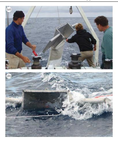
Figure 3. A manta trawl (a) being deployed from a research vessel and (b) being towed at sea to sample floating plastics.
