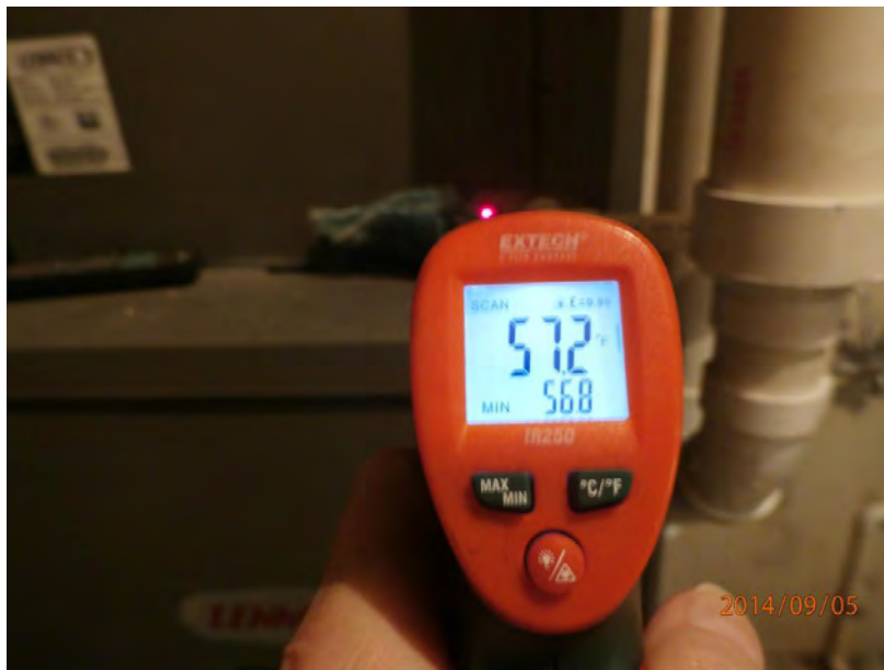
Photo shows evaporator coil cabinet at HVAC unit serving the boardroom leaking 60 degree air. Gaps around much of the edge of this access panel were leaking on almost every unit.
