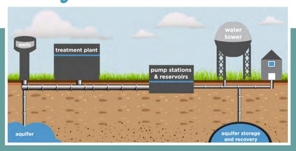
Columbia's water is pumped from 15 wells that tap an alluvial aquifer in McBaine, Mo. Softened, filtered and disinfected water is pumped from the treatment plant to reservoirs at Columbia's three pump stations. The water is then pumped throughout the city to consumers. It is stored at towers and reservoirs for times of high demand or for fire fighting.
