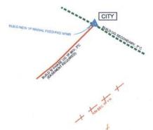
BUILD NEW PADMOUNTED SINGLE PHASE TRANSFORMER, FEED TRANSFORMER WITH NEW UG 8KV CIRCUIT IN 3" CONDUIT, USE TRANSFORMER TO FEED NEW UG 120/240V CIRCUITS IN 3" CONDUITS.
